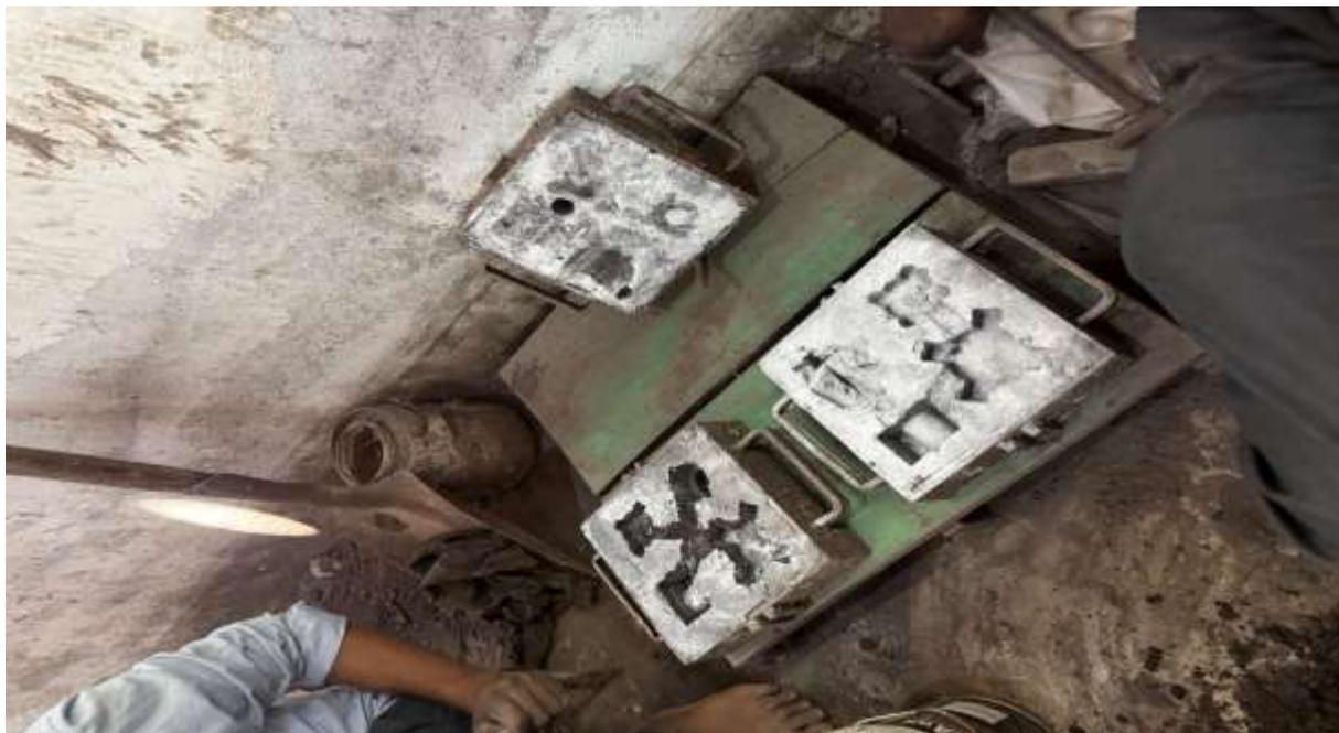
Preparation of Mould using Cope and Drag Box
