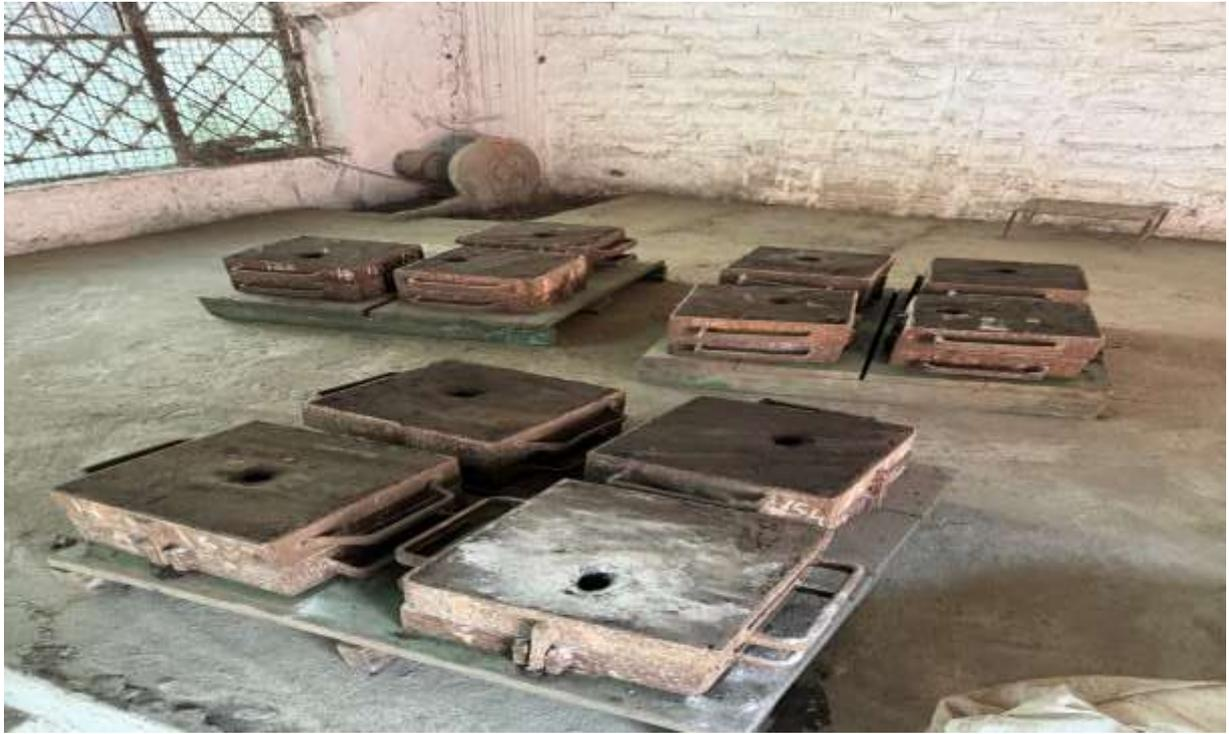
Mould ready for Pouring the Molten Metals to produce Casting
